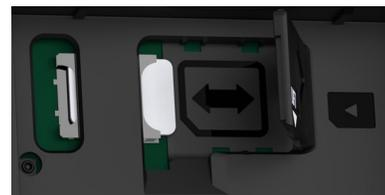
10. Carefully slide the SIM card out of the SIM card slot.
