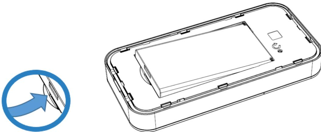
9. Lift the SIM access tab by placing a fingernail underneath the white arrow and lifting the tab up and to the right.
