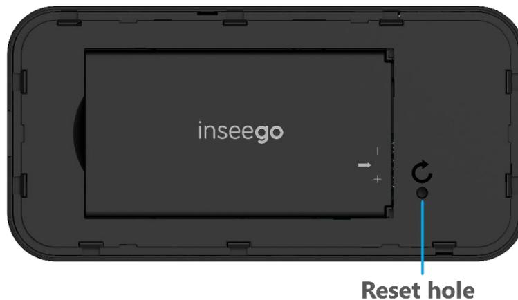
2. Place one end of an unfolded paper clip into the **Reset hole** and press until the screen displays **MiFi Resetting** (about five to six seconds). Your MiFi restarts with factory settings.
