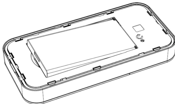
3. Align the gold contacts on the new battery with the gold contacts on the MiFi and gently slide the battery into place.
